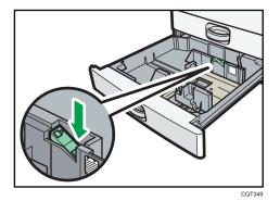
3. While pressing down the release lever, slide the side fences outward.
